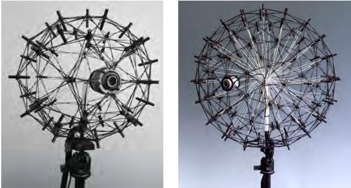
Fig. 5: Spherical acoustically transparent arrays with 48 channels and 120 channels and a built-in video camera
