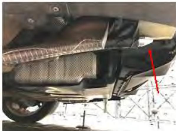
Figure 6: VVS (red arrow) to measure the transfer functions [12].
