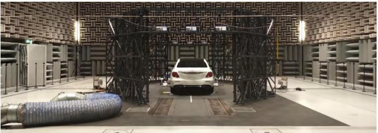
Figure 5: Car placed on the dyno surrounded by the microphone array for HIBF and the two microphone lines for simulated pass-by (at the left and right wall) [12].
