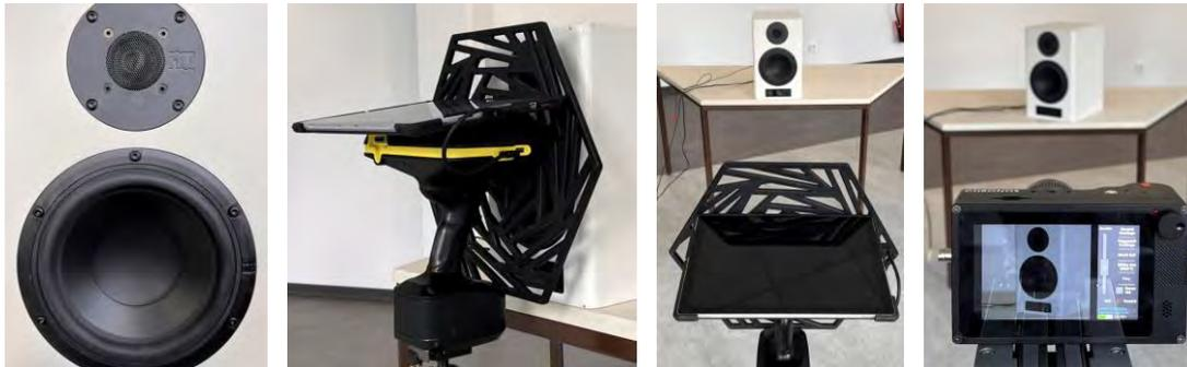
Figure 8: Speaker (left), Acoustic measurements (center), high-speed camera setup (right).
