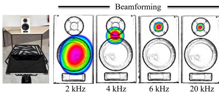
Figure 13: Beamforming (Power Beamforming [7], functional 16, 1 dB dynamic, Sound Pressure)
