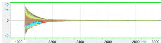
Figure 2: Acoustic response of the brake disc after single hit excitation with a metal tip.
