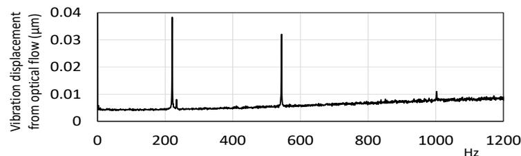
Figure 5: Optical response spectrum of the brake disc after single hit excitation with a metal tip.
