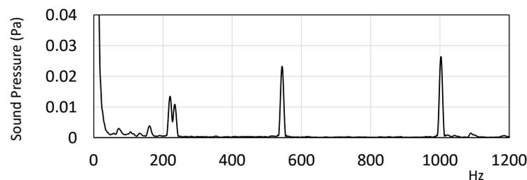
Figure 3: Acoustic response spectrum of the brake disc after single hit excitation with a metal tip.
