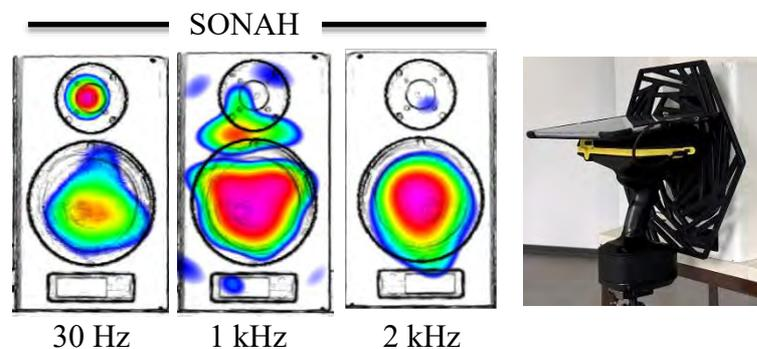
Figure 12: Acoustic holography (SONAH, 12 dB dynamic, Particle Velocity)
