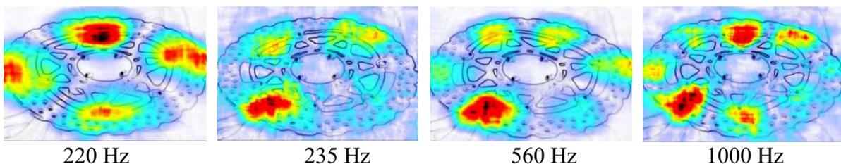
Figure 6: Frequency operating deflection shapes (ODS) based on high-speed camera recordings.
