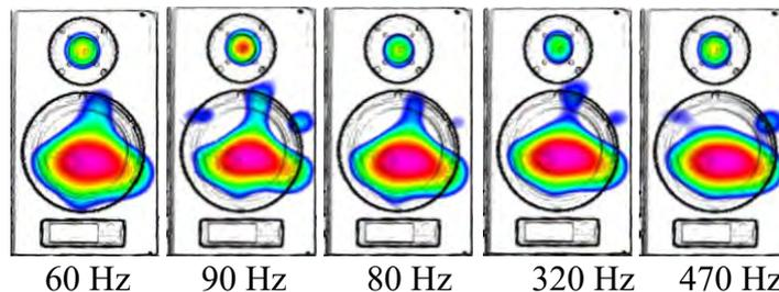
Figure 9: Acoustic holography (SONAH, 12 dB dynamic, particle velocity)
