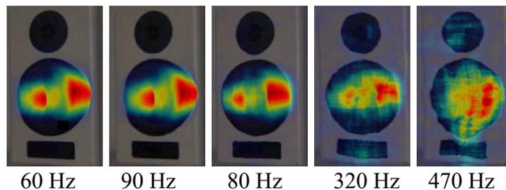
Figure 10: Frequency ODS based on high-speed camera recordings.
