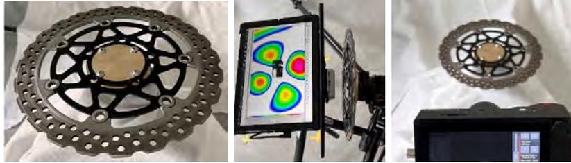
Figure 1: Rigidly mounted brake disc (left), Acoustic holography measurement (center), high-speed camera setup (right).
