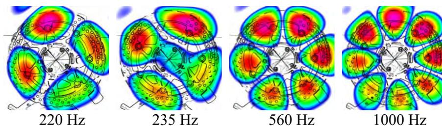
Figure 4: Mode shapes based on acoustic holography (SONAH, 20 dB dynamic, particle velocity).
