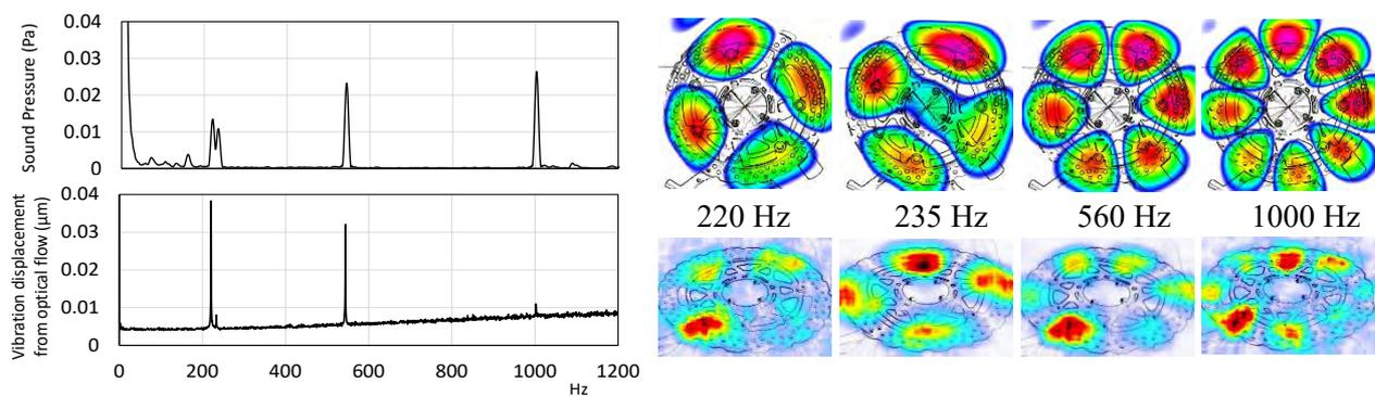
Figure 7: Comparison of spectral content and vibration shapes.
