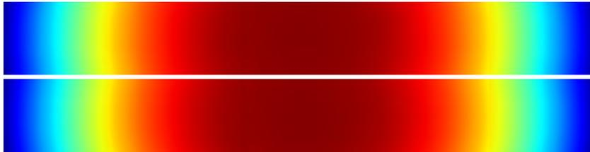
Figure 11: Pressure magnitude (12 dB), single smooth spherical piston,  $f = 1000$  Hz, simulation of degree 120 (top) and SIFAH reconstruction of degree 25 (bottom)
