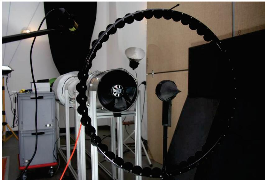
Figure 3 – Acoustic Camera measurements on the test stand
