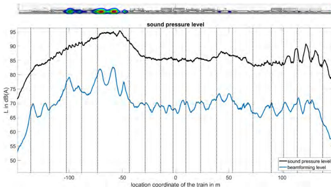
Figure 6: Comparison between sound pressure level and beamforming level of a freight train
