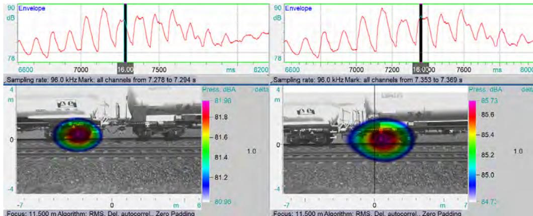
Figure 5: Examples of sound radiation of two closely spaced wheel flats of a freight train
