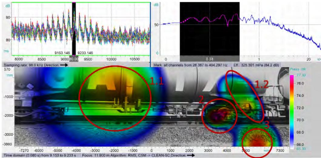
Figure 8: Low frequency sound emission on a tank wagon near an axle with a wheel flat
