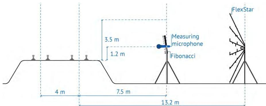
Figure 2: Measurement set-up; the "Fibonacci" array was placed 10 m away from the "FlexStar" array along the track
