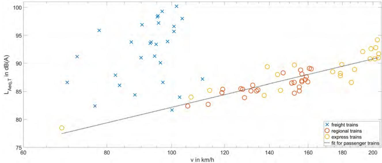
Figure 3: Total pass-by level  $L_{Aeq,T}$  as a function of the average pass-by speed
