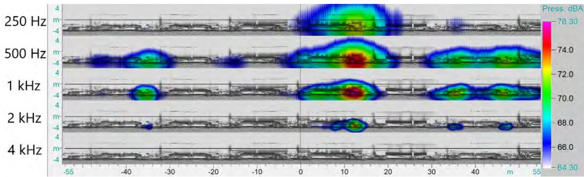
Figure 7: Pass-by evaluation of a section of a freight train for different octave bands with the same dynamic range
