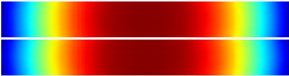
Figure 10: Pressure magnitude (12 dB), single smooth spherical piston, f = 500 Hz, simulation of degree 120 (top) and SIFAH reconstruction of degree 35 (bottom)
