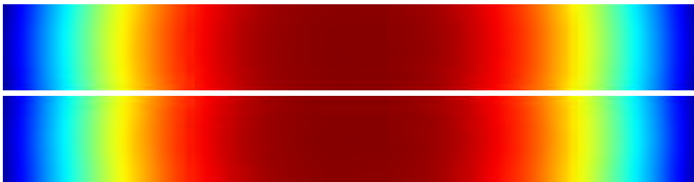
Figure 11: Pressure magnitude (12 dB), single smooth spherical piston, f = 1000 Hz, simulation of degree 120 (top) and SIFAH reconstruction of degree 35 (bottom)
