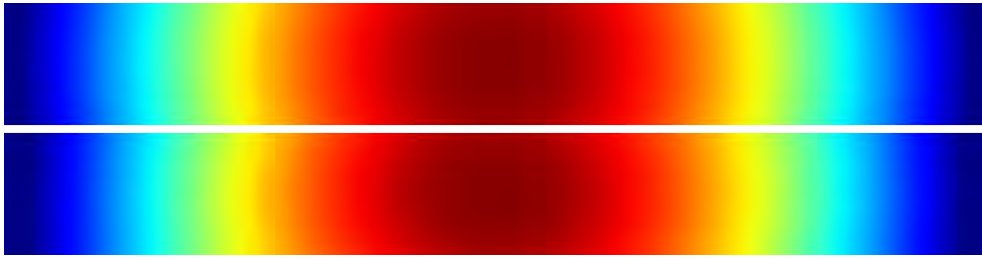
Figure 9: Pressure magnitude (12 dB), single smooth spherical piston, f = 250 Hz, simulation of degree 120 (top) and SIFAH reconstruction of degree 35 (bottom)
