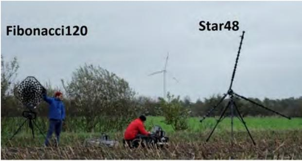
**Figure 6:** Picture of a full measurement setup consisting of both arrays, data acquisition system and computer
