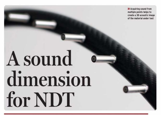
Acoustic cameras bring a new dimension to non-destructive testing (NDT) by adding sound to visual images in the hunt for defects in large composite aerospace structures
