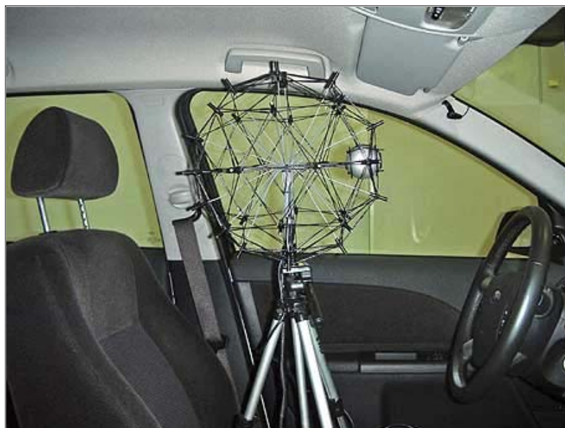
GFal's Acoustic Camera spherical array is one of several products used to measure in-vehicle noise.
