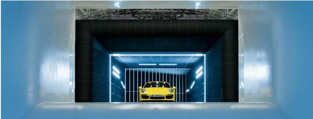
The flow channel is constricted in front of the car to attain air speeds of up to 300 km/h.
