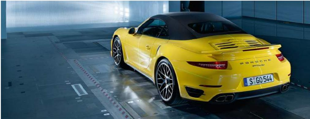
A 911 Turbo Cabriolet in the test section, or “plenum.” It is standing on a five-belt system.
