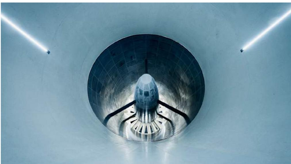
The fan's motor has an output of 7,000 kW.
