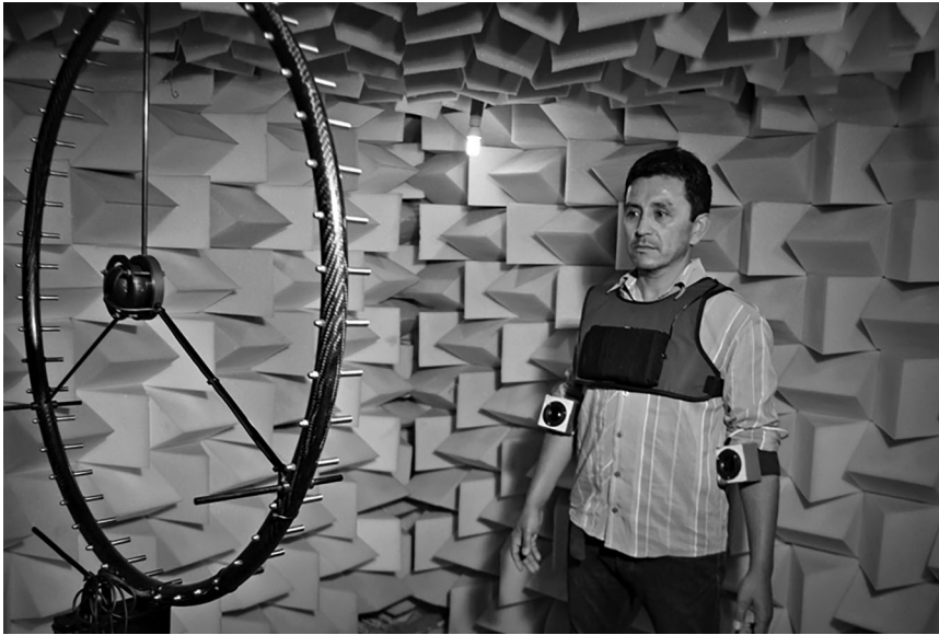
Figure 1. Acoustic camera measurements of the body-worn sound system worn by a dancer during demonstrations in an anechoic chamber.
