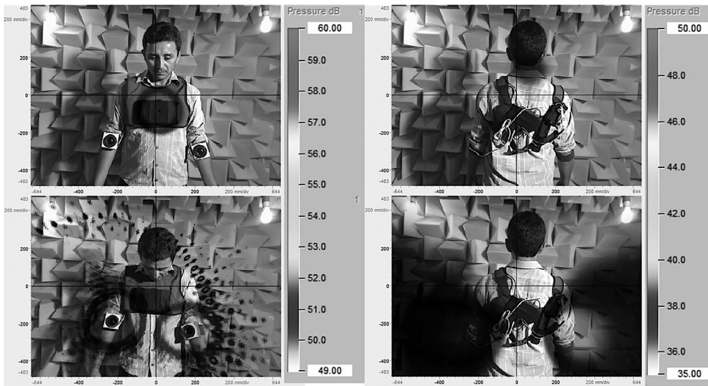
Figure 2. Measurements of the body-worn sound system during a dance demonstration carried out using an Gfai Tech Ring 48–75 ACP Acoustic Camera. Top measurements were done with the torso speaker radiating white noise, while bottom measurements were carried out with the arm speakers also radiating white noise.
