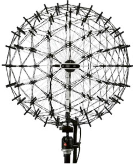
The spherical 120 channel microphone array is primarily designed for 360° sound source localization. The light carbon fiber structure ensures easy handling as well as fast and precise array positioning. The omnidirectional microphone positioning of the Sphere120 is particularly well-suited for sound source localization in enclosed spaces. Due to its acoustically transparent design, accurate measurements are carried out without influencing the sound field.
