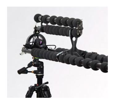
The Star48 array is our largest preconfigured array and particularly suitable for outdoor measurements of large objects. The lightweight folding aluminum body of the array ensures a stable and safe setup by just one person.
