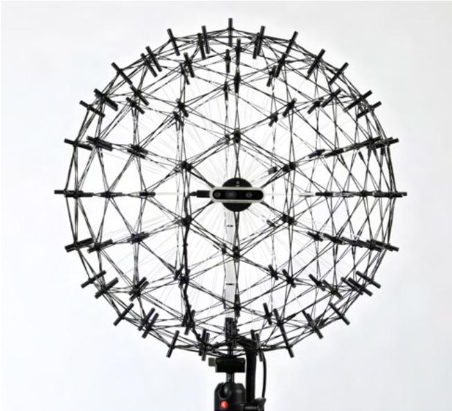
The spherical 120 channel microphone array is primarily designed for 360° sound source localization. The light carbon fiber structure ensures easy handling as well as fast and precise array positioning. The omnidirectional microphone positioning of the Sphere120 is particularly well-suited for sound source localization in enclosed spaces. Due to its acoustically transparent design, accurate measurements are carried out without influencing the sound field.
