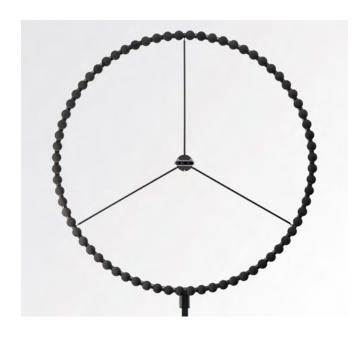
The 72 channel ring array is primarily designed for 2D measurements in acoustic laboratories, but also for outdoor measurements of larger objects. The light carbon structure ensures easy handling and quick, precise array positioning.
