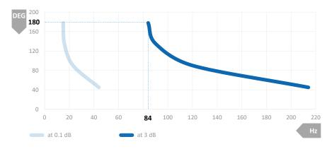
Calculation of the lowest frequency (Hz) at 180° opening angle (DEG) for 144 channels
