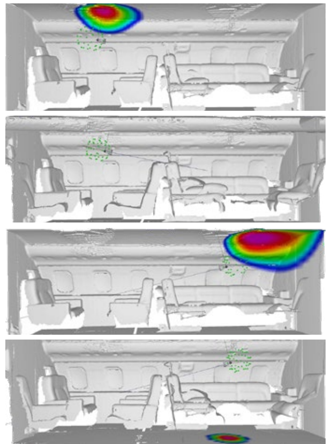
Fig. 2: Time domain results for the front and the back measurement positions
